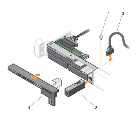
Figure 57. Removing and Installing the VGA Module
